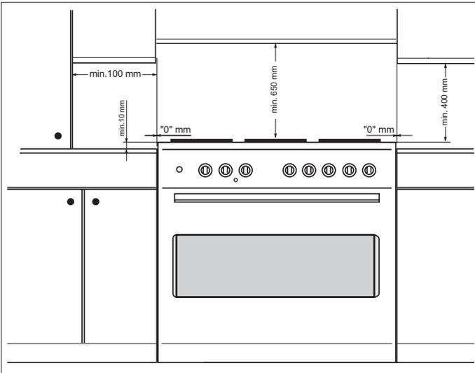
No part of any adjoining wall surface can be made of combustible materials. The protection of combustible materials required by Clause 5.12.1.1 of AS5601-2004 is the fixing of 5 mm thick ceramic tiles to the surface or attaching fire resistant material to the surface and covering with sheet metal with a minimum thickness of 0.4 mm.
