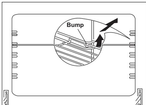
Install shelves by locating them in the horizontal guide rails on the oven walls. The raised portion of the shelf is to be facing the rear wall of the oven.
