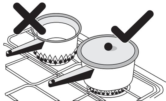
The smaller burners are for smaller pans and simmering. Make sure flames are under the pans. Using a lid will help the contents boil more quickly.
