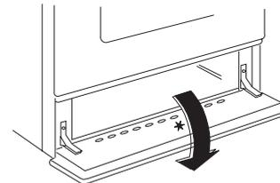
This appliance from the factory suitable for NATURAL gas but, if necessary, can be adjusted for U-LPG by authorised person.
