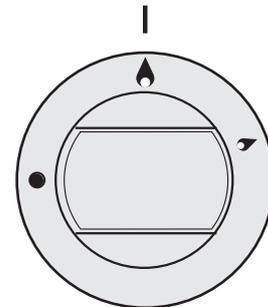
The small flame indicates the 'low position'. Turn the knob to it after the contents of a pan have boiled.
